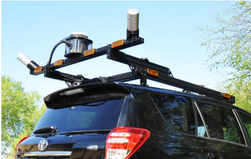
Figure 7. Configuration of two Velodyne sensors on a vehicle. (Image Credit: Mandli Communications Inc).
