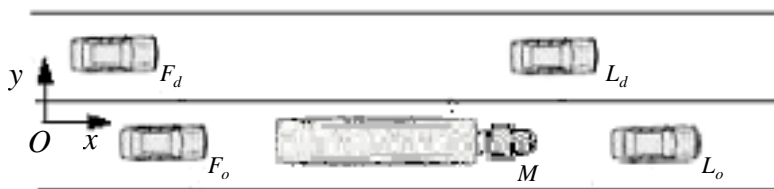
Fig. 6: Pre-lane changing configuration showing position of merging truck M .
