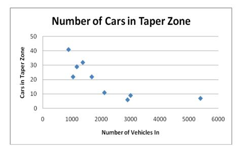
**Figure 18** Number of Vehicles in taper zone as a function of number of vehicles entering the testing zone.
