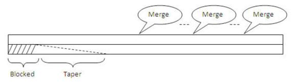
**Figure 13** Road configuration of two lane one way highway section with lane closure in ARENA module.
