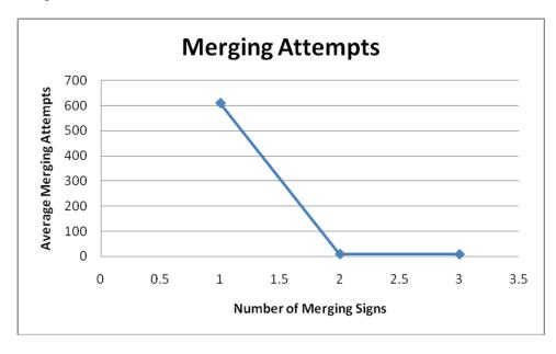
Figure 24 Merging attempts at taper end as a function of number of merging signs
