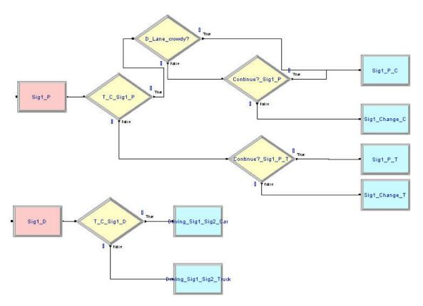
Figure 15 Model for Merging Behavior at Signal\_1
