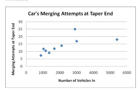
**Figure 19** Merging attempts in taper zone (a measure as risk of collision) as a function of number of vehicles entering the testing zone.
