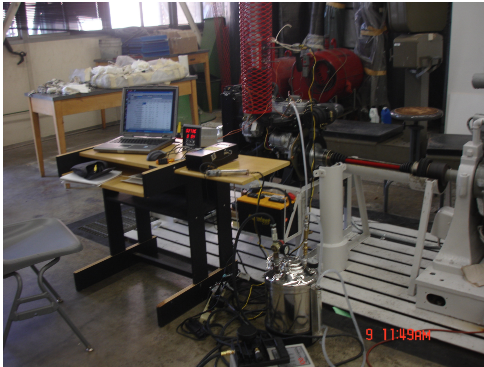
Figure 17. Diesel Engine and the SCR system.
