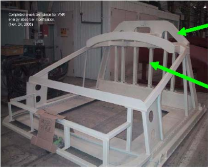
FIGURE 5 Controlled collapse cab structure prior to crush test.
