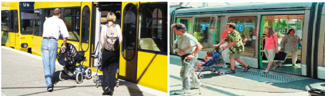
Figure 47: Roadway Platform Is Same Level with Train Floor Level
