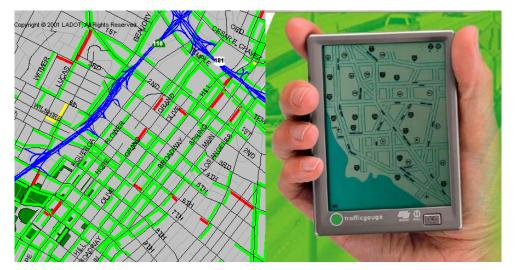
reduce delays. The information can also be fed to individual drivers through websites (see figure 8) and traffic gauge, a wireless on-time traffic information receiver (See figure 9).
