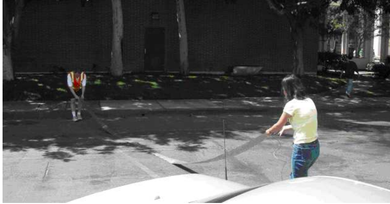
Figure 1: Deployment of a narrow inductive loop for a blade sensor.
