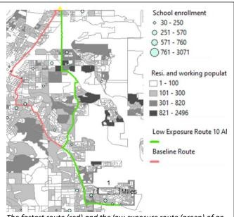
The fastest route (red) and the low exposure route (green) of an example truck trip. Compared to the baseline route, the low exposure route would take less than a minute longer, but would reduce community exposure to PM2.5 and NOx by 73% and 31%, respectively. It would also reduce CO2 emission by 9%.
