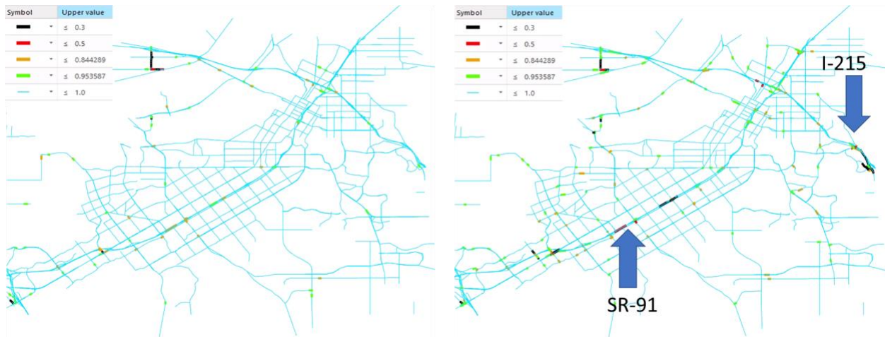
Figure 13. Link speeds during 10 AM in the car-only scenario [left] and the car & truck scenario [right]
