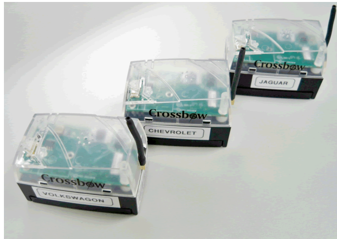
FIGURE 6 Crossbow Technologies Wireless Motes Used in Testbed
