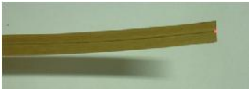
Fig. 18 Section of distributed fiber optic sensor
